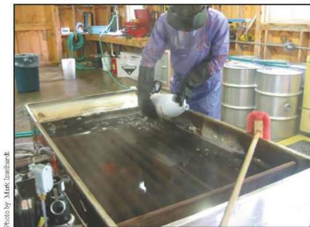
Cleaning pans with the appropriate personal protective equipment, including chemical-resistant gloves, protective clothing and a faceshield.
